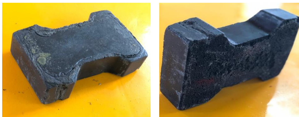
Figure 6. Product of the recycled plastic pavement fabrication process (70% LDPE, 30% sand).
