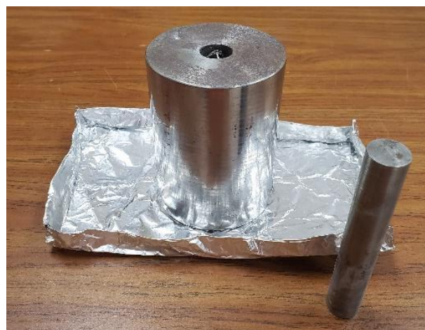
Figure 5. Preheated die filled with pellets.
