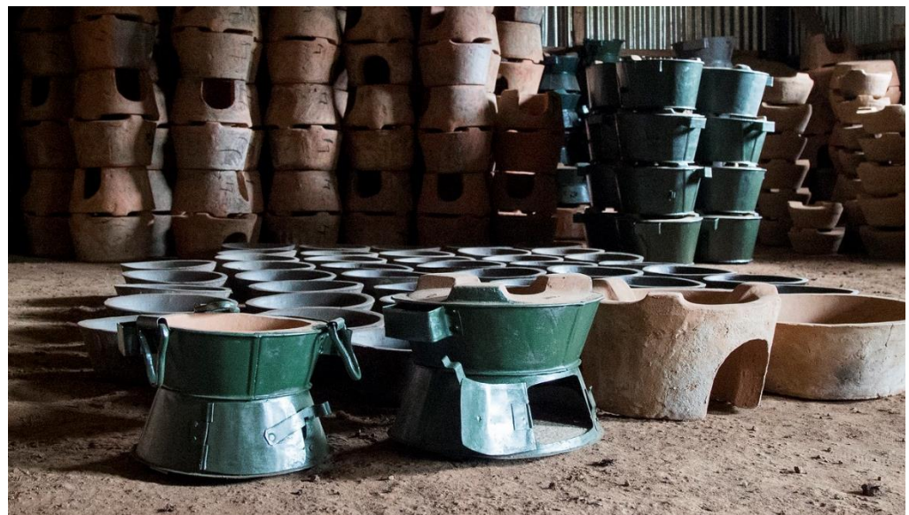
Figure 4. Artisanal African stove that is designed to burn wood, charcoal, or carbonized waste pellets [38].
